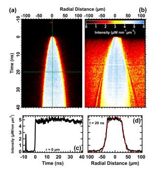
FIG. 1. Time-resolved radial cross section of a spark discharge in 42 bar (a) and 10 bar (b) Xe. In (b), a backlight renders the emitted shock wave visible. Temporal (c) and radial (d) lineouts, whose position is indicated by the green dotted lines in (a), reveal brightness saturation occurring both in time and space. A weak femtosecond laser pulse initiates the discharge, indicated by emission at -8 ns in (a) and (c). The red-dashed curve in (d) is the best-fit super-Gaussian.
