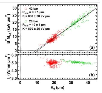
FIG. 5. Scatter plots of (a)  $B^2 M_{Xe}$  and (b) the brightness of the spark channel vs the initial plasma radius for individual discharges at 20 and 40 bar.  $B^2 M_{Xe}$  is proportional to  $(R_0 - R_{\min})$  and is pressure independent, while the surface brightness is independent of both spark size and pressure.
