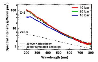
FIG. 3. Absolute spectral intensity of Xe discharges at 3 ns for various static pressures. Spectral saturation throughout the measured spectrum occurs for pressures > 10 bar and is well fit to a 29 000 K blackbody spectrum (dotted). Simulated spectra (dashed) at 20 bar were calculated for various levels of ionization (Z=0.3 and 2) using Eq. (7) at  $T_{\rm sat}=29000$  K and  $l=40~\mu{\rm m}$ .
